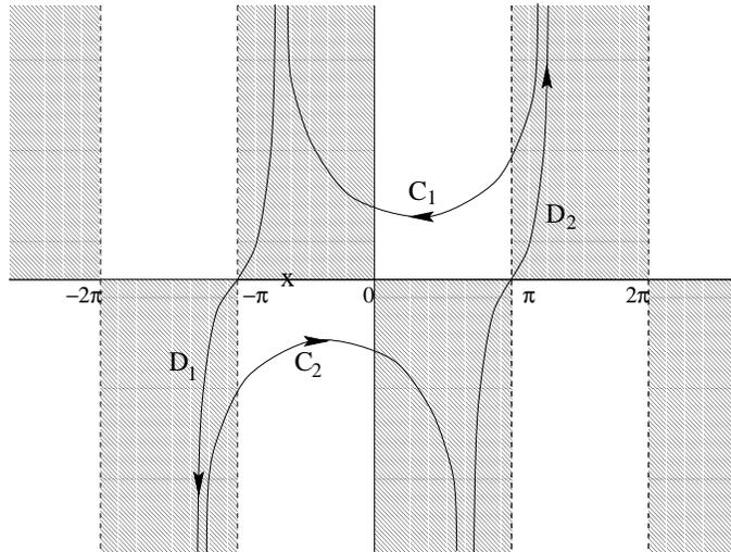
**Figure 38.2:** The contour in the complex  $\beta$  plane. The pole is at  $\beta = -\psi$  (marked by  $\times$  in the figure) and the integrand approaches zero in the shaded regions as the magnitude of the imaginary part of  $\beta$  approaches infinity.
