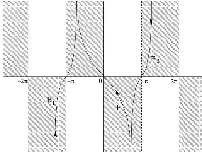
**Figure 38.3:** The contour used to evaluate the diffractive field after the contribution of possible poles has been explicitly evaluated. The curve  $F$  is traversed twice in opposite directions and has no net contribution.
