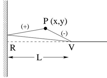
order in  $y$  the lengths of the two geometric paths connecting  $P$  and  $V$  are  $d_{\pm} = (L \pm x) + y^2 / (L \pm x)^2 / 2$  so that the phase factor  $ik(d_+ + d_-)$  equals  $2ikL +iky^2 / (L^2 - x^2)$ . The trace integral involves integrating over all points  $P$  and is
