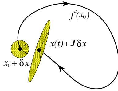
**Figure 4.2:** The Jacobian matrix  $J^t$  maps an infinitesimal displacement at  $x_0$  into a displacement rotated and sheared by the linearized flow Jacobian matrix  $J^t(x_0)$  finite time  $t$  later.
