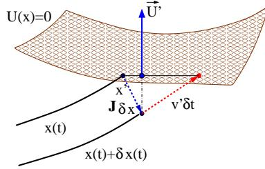
**Figure 4.9:** If  $x(t)$  intersects the Poincaré section  $\mathcal{P}$  at time  $\tau$ , the nearby  $x(t) + \delta x(t)$  trajectory intersects it time  $\tau + \delta t$  later. As  $(U' \cdot v' \delta t) = -(U' \cdot J \delta x)$ , the difference in arrival times is given by  $\delta t = -(U' \cdot J \delta x)/(U' \cdot v')$ .
