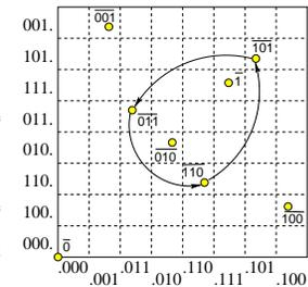
**Figure 12.9:** Kneading danish pastry: symbol square representation of an orientation preserving once-folding map obtained by fattening the Smale horseshoe intersections of figure 12.4 (e) into a unit square. Also indicated: the fixed points  $\bar{0}, \bar{1}$ , and the 3-cycle points  $\{011, 110, 101\}$ . In the symbol square the dynamics maps rectangles into rectangles by a decimal point shift.
