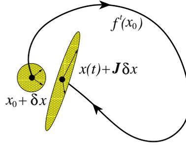
**Figure 17.5:** The symmetric matrix  $\mathbf{J} = (J')^T J'$  maps a swarm of initial points in an infinitesimal spherical neighborhood of  $x_0$  into a cigar-shaped neighborhood finite time  $t$  later, with semiaxes determined by the local stretching/shrinking  $|\Lambda_i|$ , but local individual trajectory rotations by the complex phase of  $J'$  ignored.
