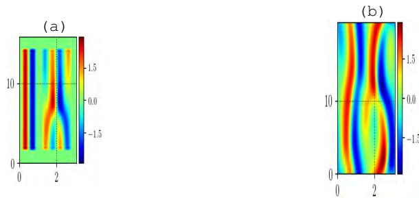
Figure 18.13: (a) Initial spatiotemporal field for the one-by-two symbolic block given by (1.83) (b) Invariant 2-torus resultant from numerically converging (a), [L_b, T_b] = [3.13 \dots, 20.84 \dots]
