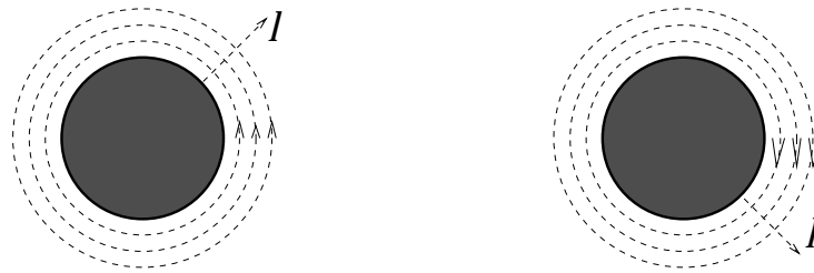
Figure 33.2: Left- and right-handed diffractive creeping paths of increasing mode number \ell for a single disk.
