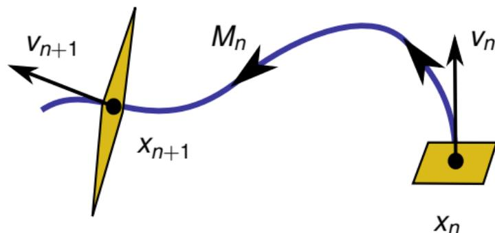
$$x_{n+1} + z_{n+1} = f(x_n) + M_n z_n, \quad M_{ij} = \partial f_i / \partial x_j$$
