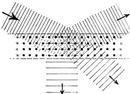
**Fig. 21.2** The Davisson–Germer experiment. A beam of electrons of 3-momentum  $\mathbf{p}$  encounters a material of periodic crystalline structure. Scattering or reflection occurs when the atomic pattern matches with that of the electrons, these being regarded as waves with a wavelength  $\lambda$  related to the magnitude of the momentum  $p$  according to  $\lambda = h/p$ , where  $h$  is Planck’s constant.
