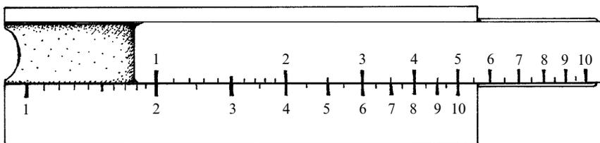
**Fig. 5.6** Slide rules display numbers on a logarithmic scale, thereby enabling multiplication to be expressed by the adding of distances, in accordance with the formula  $\log_b(p \times q) = \log_b p + \log_b q$ . (Multiplication by 2 is illustrated.)
