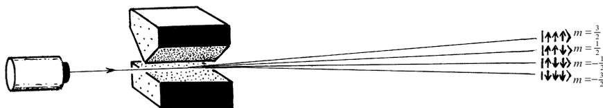
**Fig. 22.15** Stern–Gerlach apparatus, used to measure the ‘ $m$ -value’ of an atom’s magnetic moment (coupled to its spin). The atoms pass through a strongly inhomogeneous magnetic field, deflecting their paths slightly differently for each  $m$ -value.
