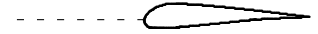
A static airfoil in an airstream coming in horizontally from the left. The shown streamline (dashed) ends in the forward stagnation point.
