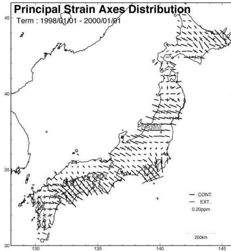
Figure 7.3. Principal strain axis distribution for ground displacements in Japan, determined by GPS over two years. Only the two horizontal axes are shown with lengths proportional to the magnitude of the eigenvalues. The black axes (running mainly southeast-to-northwest) indicate contraction and the gray extension. Geography & Crustal Dynamics Research Center (Permission to be obtained).
