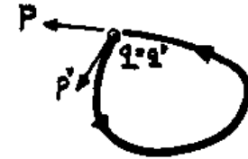
Figure 34.1: A returning trajectory in the configuration space. The orbit is periodic in the full phase space only if the initial and final momenta of a returning trajectory coincide as well.
