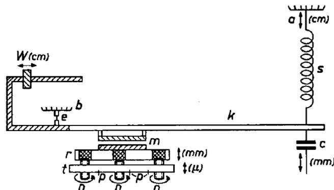
FIG. 4: Sparnaay developed an apparatus that counterbalanced a plate over another plate using a spring and a wire attached to fixed mounts. The capacitance was then measured between two plates mounted below the spring. Alignment of parallel surfaces was intricate and done using several micrometers.
