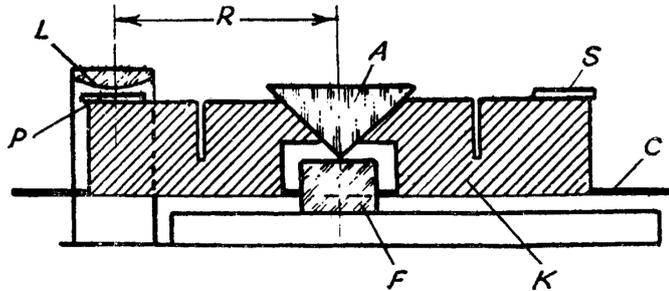
FIG. 3: Derjaguin investigated the Casimir force with his collaborators Brikosova and Lifshitz using a beam balance with a quartz lens and a quartz plate as shown above. Here L is the spherical lens. P is the plate it interacts with. A is a prism that serves as a pivot and F is the fulcrum it rests on. S is a mirror and C is a counterweight.
