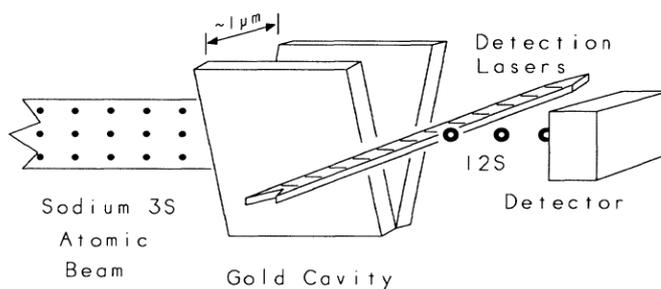
FIG. 5: Sukenik constructed a device which passed sodium ions through a channel between two gold plates. The ions at a height were excited upon exiting and impinged on a device that would measure them.
