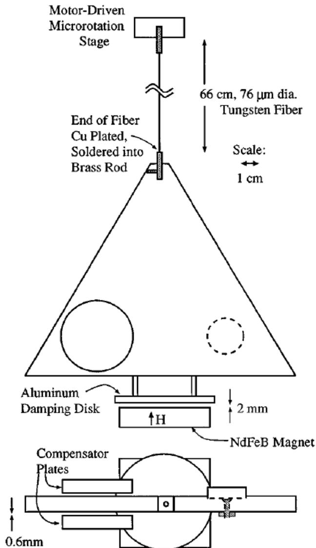
FIG. 6: Lamoreaux constructed a pendulum, which would be brought into proximity of a plate at one end. Force was measured by the capacitance between the pendulum and two plates on either side of it. The range was dependent of a feedback system, which operated a series of piezoelectric devices designed to keep the capacitance the same on both sides.
