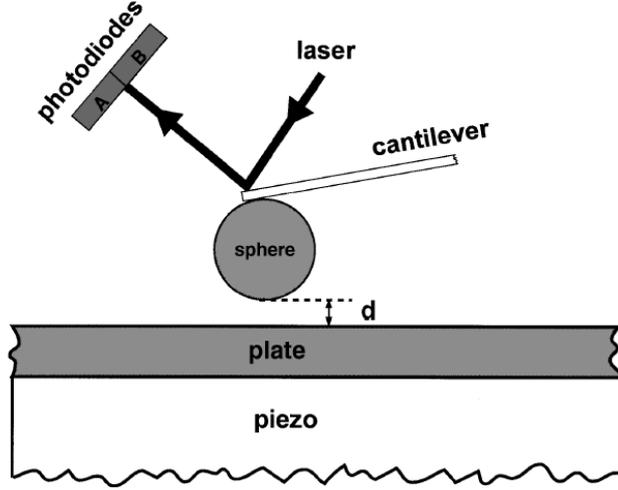
FIG. 7: Here we can see the bead attached to an AFM tip as a cantilever. The laser impinges on the cantilever surface and reflects to a pair of photodiodes whose intensities are compared to determine the amount of deflection of the cantilever.
