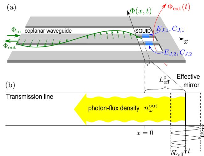
FIG. 8: Here we see the coplanar waveguide that terminates with a SQUID to have a variable boundary. The size of the boundary is controlled by  $\phi_{ext}(t)$ . By measuring the photon flux density they were able to determine that photons were being excited by vacuum fluctuations.
