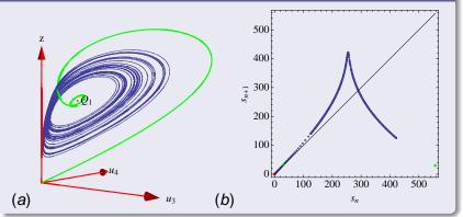
(a) The unstable manifold connection from the equilibrium  $E_0$  at the origin to the strange attractor controlled by the rotation around the reduced state space image of relative equilibrium O:
