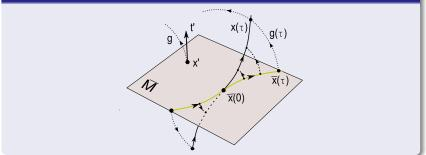
Slice  $\overline{\mathcal{M}}$  through the slice-fixing point x', normal to the group tangent t' at x', intersects group orbits (dotted lines). The full state space trajectory  $x(\tau)$  and the reduced state space trajectory  $\overline{x}(\tau)$  are equivalent up to a group rotation  $g(\tau)$ .
