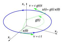
relative equilibrium (traveling wave, rotating wave)  $x_{TW}(\tau) \in \mathcal{M}_{TW}$ : the dynamical flow field points along the group tangent field, with constant 'angular' velocity *c*, and the trajectory stays on the group orbit
