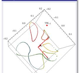
Relative periodic orbit intersects a hyperplane slice in 3 closed-loop images of the relative periodic orbit and 3 images that appear to connect to a closed loop.
