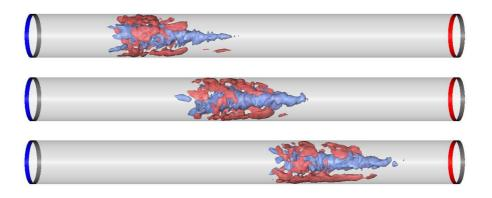
Figure 4. Three snapshots of a turbulent flow in a pipe at Re = 1825, moving from left to right. The snapshots are separated in time by  $20D/u_{cl}$  with  $u_{cl}$  the centerline velocity. The red and blue regions indicate isosurfaces of downstream velocities somewhat faster or slower than the parabolic laminar profile. The aspect ratio is not shown to scale: the pipe is 50 diameters long. From (Eckhardt & Schneider 2008).
