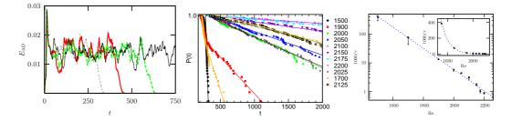
**Figure 2.** The energy traces in a turbulent section as a function of time show turbulent dynamics followed by a decay back to the laminar profile. When collected over many initial conditions, exponential distributions of life times result (middle). The characteristic lifetimes increase rapidly with Reynolds number (right).
