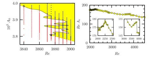
**Figure 3.** The boundary between laminar and turbulent (left) for a specific perturbation and the scaling of the boundary with Reynolds number. The insets on the right show modulations in the scaling curve connected with the folds on the left. From (Schneider, Eckhardt & Yorke 2007).
