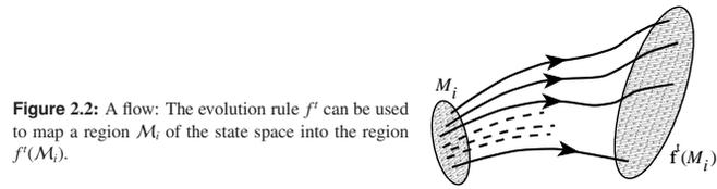
**Figure 2.2:** A flow: The evolution rule  $f^t$  can be used to map a region  $M_i$  of the state space into the region  $f^t(M_i)$ .
