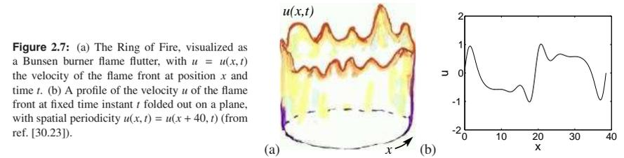
**Figure 2.7:** (a) The Ring of Fire, visualized as a Bunsen burner flame flutter, with  $u = u(x, t)$  the velocity of the flame front at position  $x$  and time  $t$ . (b) A profile of the velocity  $u$  of the flame front at fixed time instant  $t$  folded out on a plane, with spatial periodicity  $u(x, t) = u(x + 40, t)$  (from ref. [30.23]).
