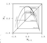
**Figure 3.6:** The strange attractor and an unstable period 7 cycle of the Hénon map (3.17) with a = 1.4, b = 0.3. The periodic points in the cycle are connected to guide the eye. (from K.T. Hansen [15.23])
