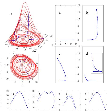
**Figure 3.2:** (Right:) a sequence of Poincaré sections of the Rössler strange attractor, defined by planes through the z axis, oriented at angles (a)  $-60^{\circ}$  (b)  $0^{\circ}$ , (c)  $60^{\circ}$ , (d)  $120^{\circ}$ , in the x-y plane. (Left:) side and x-y plane view of a typical trajectory with Poincaré sections superimposed. (R. Paškauskas)
