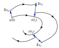
**Figure 17.4:** A long-time numerical calculation of the leading Lyapunov exponent requires rescaling the distance in order to keep the nearby trajectory separation within the linearized flow range.
