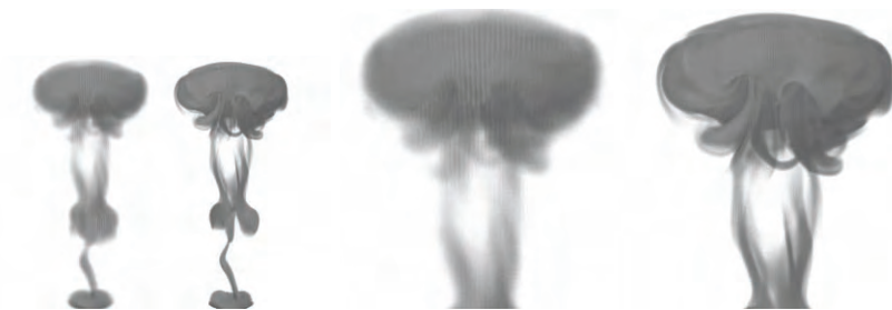
Fig. 1. Left pictures: volume rendering comparison of a low (left pictures) and high (right pictures) resolution of scalar in an under-resolved jet. The right pictures are a close-up view of the top part of the jet.
