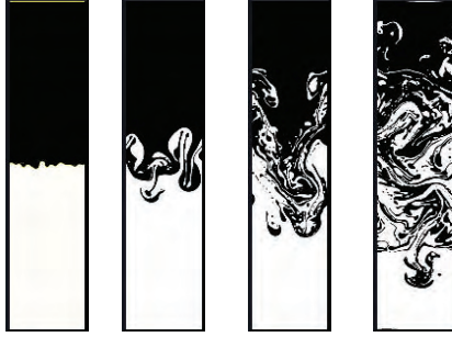
Fig. 1. Two-color snapshots of density field at different times. White (black) corresponds to a light (heavy) fluid. Our system consists of two immiscible, incompressible fluids having different densities in the presence of gravity. At initial time, the system is at rest in unstable configuration. If a disturbance is imposed on the interface separating the two fluids, the instability develops.
