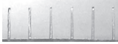
Fig. 2. A row of micro-pillar shear-stress sensors. If the sensors are aligned in spanwise direction ( z ) it is possible to obtain a temporal correlation between \partial\tau_x/\partial z and \tau_z . Note that in the present investigation the sensors are placed further apart than in the picture. Their spacing roughly corresponds to twice the pillar height.
