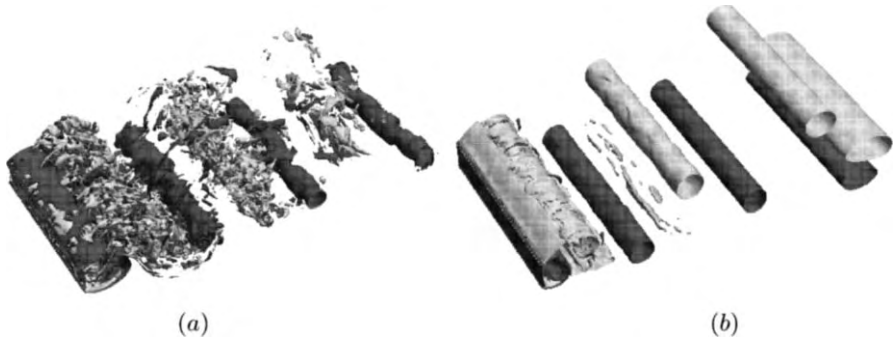
Fig. 2. Iso-surface plot of spanwise vorticity. (a) Ro_g = 1 , (b) Ro_g = 0.16
