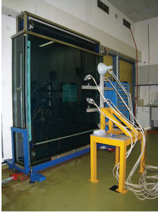
Fig. 1. Plane Couette facility setup. Inside a 2 \times 2 \times 0.25 \text{ m}^3 water tank an endless belt of 1.6 m width is controlled by two large driving drums that measure 219 mm in diameter. The optically accessible measuring domain with sheared flow is 1.6 \times 1.6 \times 0.03 \text{ m}^3 .
