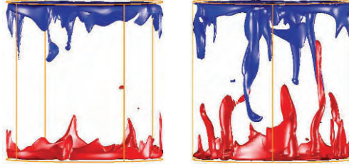
Fig. 3. 3D visualization of the temperature isosurfaces in the cylindrical sample of \Gamma = 1 at 0.65\Delta (red) and 0.35\Delta (blue), for Pr = 6.4 , Ra = 10^8 and Ro = \infty (left) Ro = 0.30 (right). The snapshots were taken in the respective statistically stationary regimes [2].
