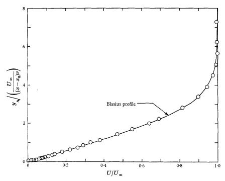
FIGURE 3*a*. Test of the hot wire in a laminar flow. O, hot-wire data;  $x_0$ , effective origin found by fit.
