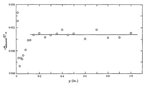
FIGURE 5b. Determination of the wall shear stress by the cross-plot method. Station 6,  $dP/dx < 0. v^*/U_{\infty} = 0.0508, U_{\infty} = 0.462 \text{ ft./sec}; v^* = 0.023 \text{ ft./sec}.$
