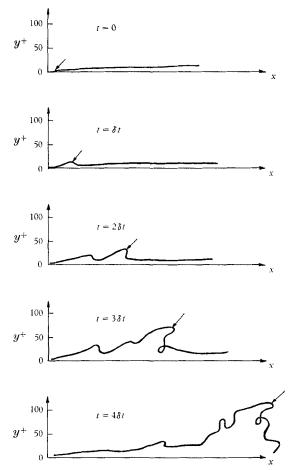
FIGURE 15. Dye streak breakup; illustration as seen in side view.
