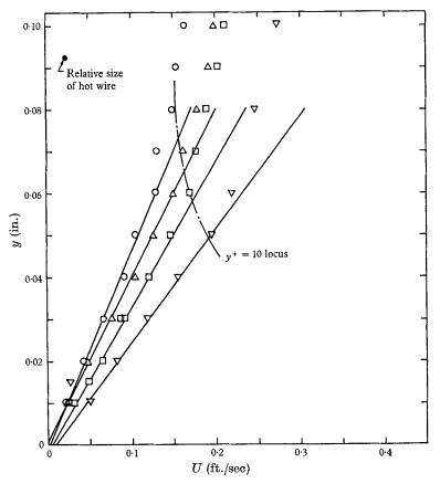
FIGURE 5*a*. Determination of the wall shear stress by the wall-slope method.  $\nabla$ , station 6;  $\Box$ , station 8;  $\triangle$ , station 11;  $\bigcirc$ , station 15; dP/dx < 0.
