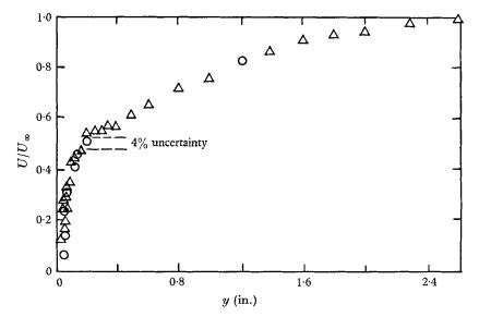
FIGURE 3b. Comparison of mean velocity data from hot-wire and bubble techniques. Station 10,  $dP/dx \ge 0$ .  $\triangle$ , hot wire;  $\bigcirc$ , hydrogen bubble.
