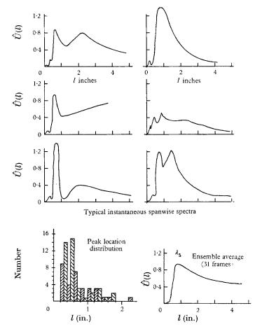
FIGURE 14. Typical instantaneous and average spanwise spectra.  $dP/dx \ge 0$ ,  $y^+ \approx 2$ .
