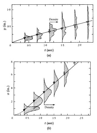
FIGURE 17. Trajectories of ejected eddies—flat plate flow. Station 10, dP/dx = 0;  $\bigtriangledown$ , averages;  $\bigcirc$ , maxima.
