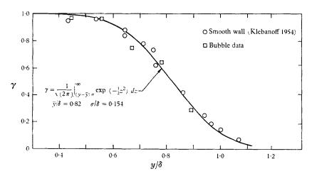
FIGURE 11. Intermittency distribution by the bubble technique.
