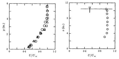
FIGURE 4. Representative checks on the two-dimensionality of the flow. Station 12,  $dP/dx \ge 0$  (worst case), y = 4.50 in.  $\bigcirc$ , z = 10 in.;  $\triangle$ , z = 7.7 in.;  $\square$ , z = 5.5 in.
