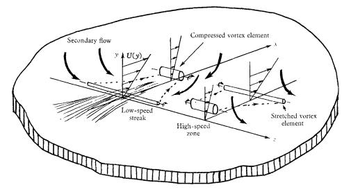
FIGURE 19a. The mechanics of streak formation.
