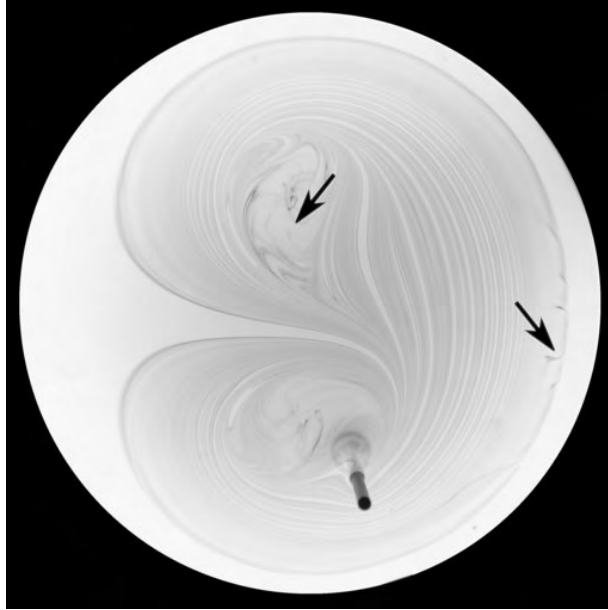
Figure 2.9: 3-D effects – In weakly stretched regions, such as the no-slip boundary or non-chaotic regions, small convection movements induce three-D effects that start spoiling the mixing pattern after about 30 periods of the stirring pattern. This is especially marked for particles close to the boundary, which are slowly advected to other parts of the domain (because of the chaotic nature of their trajectory) and contaminate the whole pattern.
