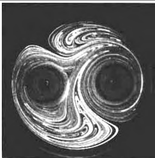
Figure 4.27: Dye homogenization experiment in a co-rotative blinking vortex, taken from Jana et al. [50]. Two cusps at the border the dye pattern reveal the presence of two parabolic points on the boundary. This is a variant of the figure-eight protocol where there is only one parabolic point on the wall.
